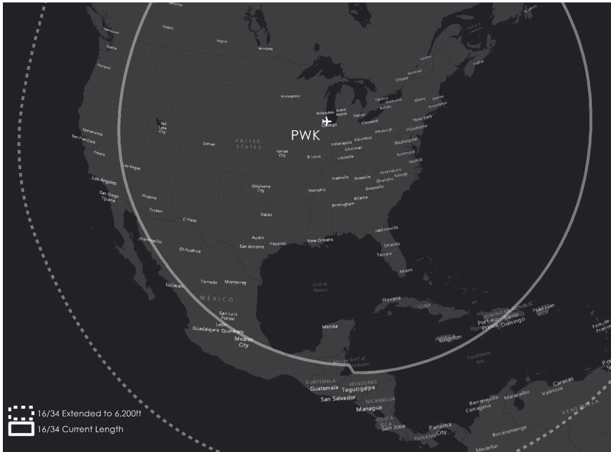
Figure 13, the payload range increase from a 6200ft runway extension with an 800XP provides significantly increased access for medium and small cabin aircraft to gain access to West Coast destinations, as well as several other Caribbean and Central American Destinations.
