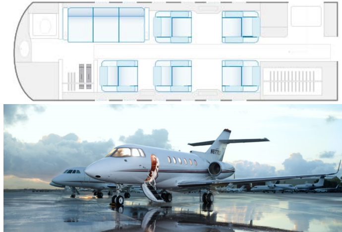
Figure 6 Hawker 800XP Seating Configuration Pictured Above, with Exterior Aircraft Image Below
