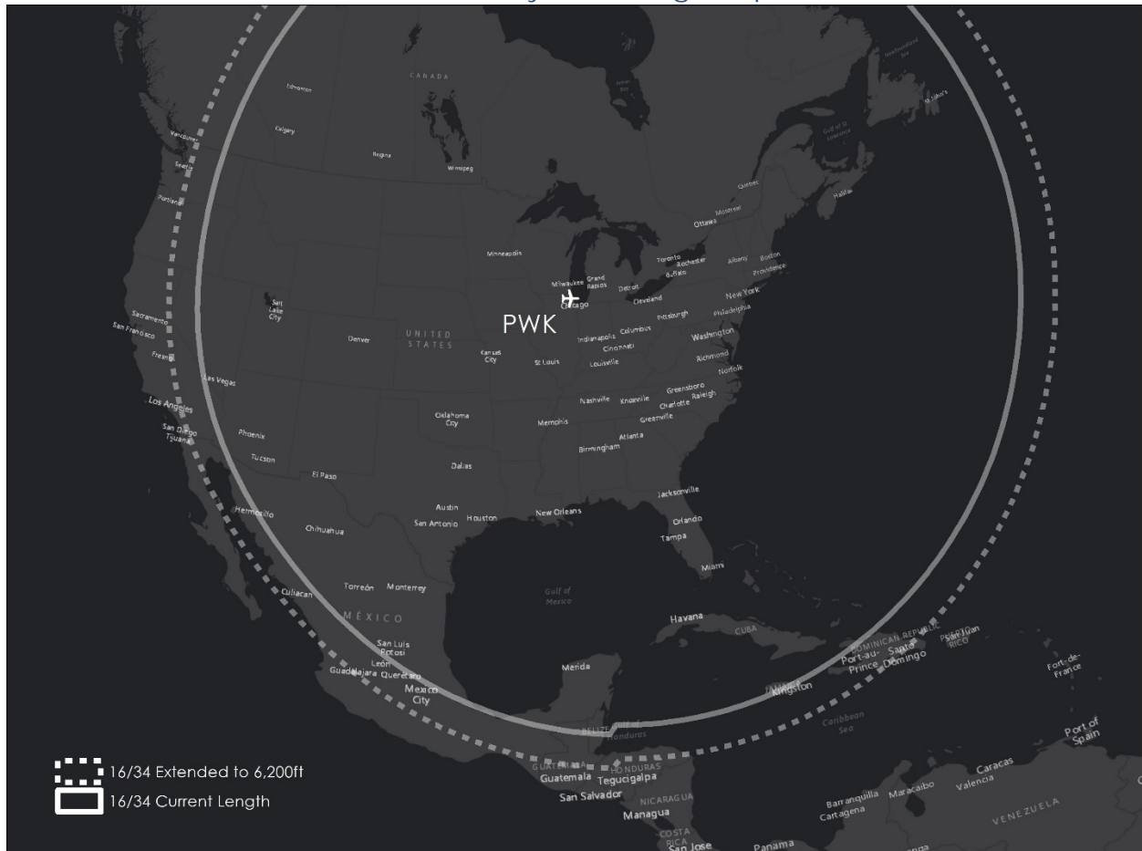
Figure 12 Payload Range Enhancement for 560XLS Between Current Runway and 6,200ft Length Runway
